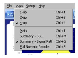
There are two views of the summary table: SSC and Signal Path. Both summary selections contain the noise and jitter measurements but not the breakdown of the measurements. The two summaries differ by displaying relevant application settings.
