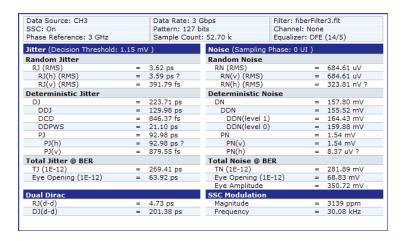
You can easily switch between summary and detailed numeric displays with the use of the numeric results button and the plot window buttons
